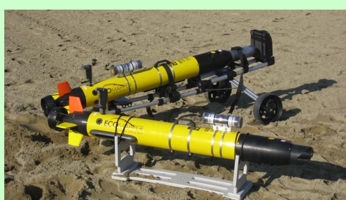
New AUVs: image + side scan sonar (100 m) and water quality (200 m)
